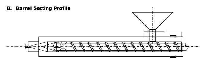
MAX 230°C/446°F 230°C/446°F 220°C/428°F MIN 190°C/374°F 190°C/374°F 180°C/356°F
